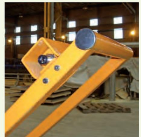
▶ Safety light beams fitted to press carriage.
