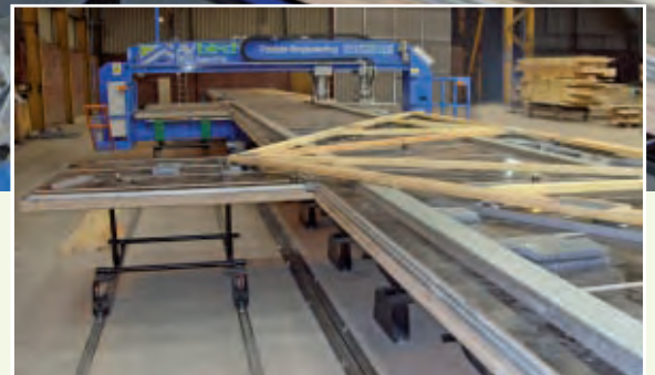
▶▶ Powered Lifters to release Truss clear from obstructions
